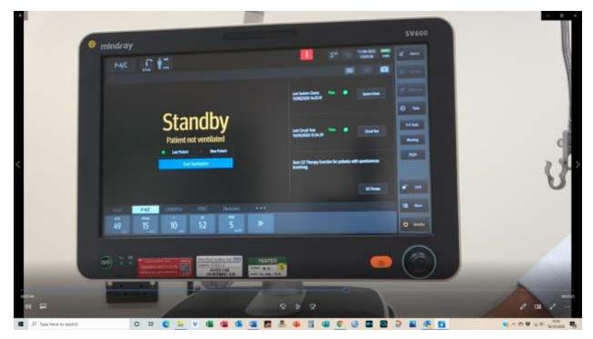
[00:08:03] So you would actually remove the old circuit, hook up the new circuit, sorry, and go just a circuit test. Go to continue and you see here the progress and that's it, then you can actually connect to the patient and go back to the actual ventilation.
