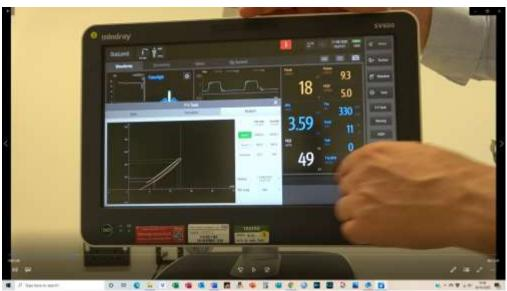
[00:02:27] All right. So, of course, first there's a warning note because it is the recruitment manoeuvre that might be quite aggressive. So what what we do here is set up the holding pressure and the time pressure in seconds to set it up to a shorter time and just like a lower pressure.
