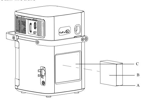
A. Latch at the bottom of the module
